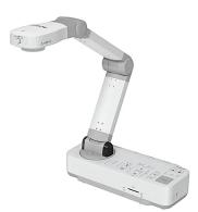
Click the power button once on the base to turn it on. Next, on the computer (Epson camera must be on before this step!), click the Start button and click on the Camera app. If the screen displays from the Owl Camera, there is an icon in the upper-right of the screen that will allow you to switch between the Owl and the Epson.
