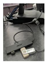
There may be a device plugged into the USB port that gives you more than one USB port. This will allow you to plug in the laser pointer dongle along with a USB Thumb drive. If the port on the monitor is not working, please see someone in the Help Desk office (which
